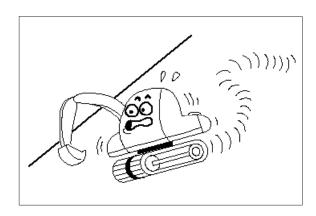
The engine angularity limits are 35 degree.
